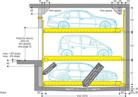
in this zone, 0% of downward/upward slope in longitudinal and cross direction
