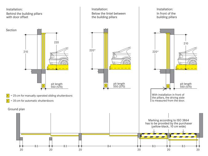
\* The lintel of 220 cm is absolutely necessary. If differing heights additional fixings are required at additional charge. If no lintel is provided, the gates need to be fitted onto a steel frame (subject to surcharges).
