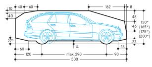
\* The total car height includes roof rail and antenna fixture and must not exceed the mentioned max. height dimension.
