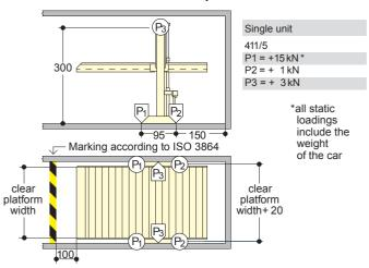
The units will be fixed on the anchor points with heavy duty anchor bolts to a depth of approx.  $10-12\ cm$ .
