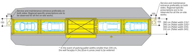
\* In the event of parking pallet widths smaller than 235 cm, the wall facades in the drive-in areas need to be widened to ensure unilateral vehicle get-in and get-out by users.
