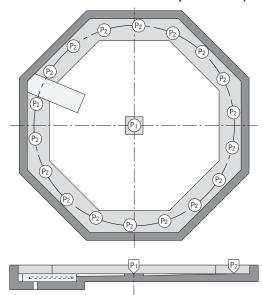
The framework construction is attached with adhesive anchors.
